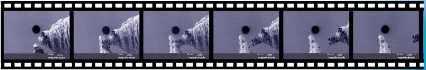
Fig. 2: Transfer of micro-particles between two Nanomanipulators by changing forces from adhesion to magnetism.
