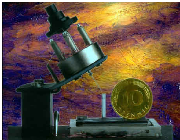
Fig. 3: A Workbench for Nanobiology, made out of a Nanomanipulator and a linear table from Klocke Nanotechnik, Aachen.
