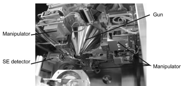
Figure 2. Photo of SEM chamber with four nanomanipulators installed around the cone of the electron gun in the center.
