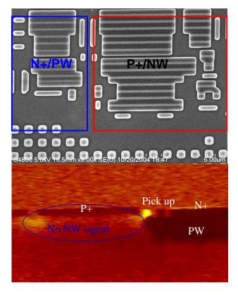
Figure 4. Junction stain shows there is no difference of contrast between N-well and P-well, which should be
