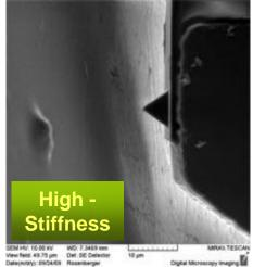
High Stiffness sensors for harder samples
