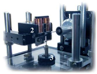
The glue is spent with a Nanomanipulator (1). The microtip is fixed in an electromagnetic holder (2), the shear force sensor is moved with the xyzpositioner (3).
